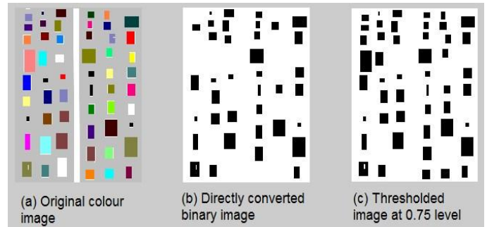
[8] Fig. 7. Comparison of directly converted binary image and thresholded binary image
